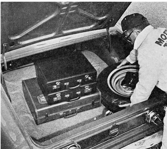
Hardtop trunk is large but has a high lip. Spare is easy to get at, yet takes up space that could be used for luggage.
