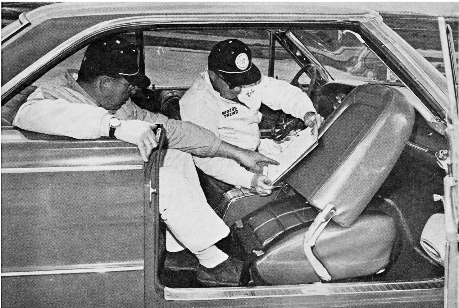
COMET'S WIDE DOORS AFFORD EASY ENTRY AND EXIT. BACK SEAT, HOWEVER, LACKS LEG ROOM AND IS TOO LOW FOR COMFORT ON LONG HAULS.
