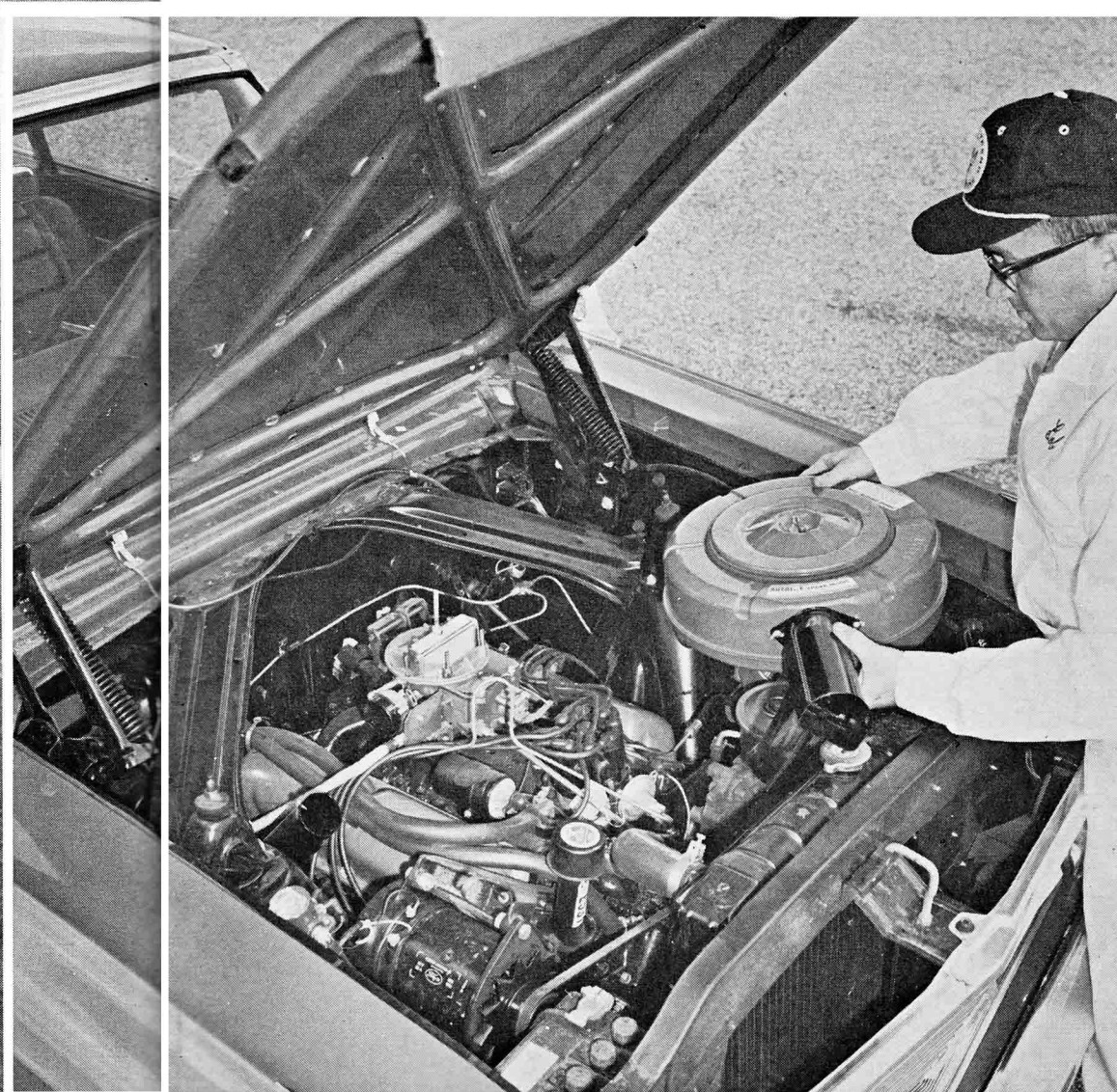
A 260-inch V-8 engine under the hood doesn't leave much room for routine maintenance. Additional struts from cowl to the fender-mounted spring housings increase rigidity.
