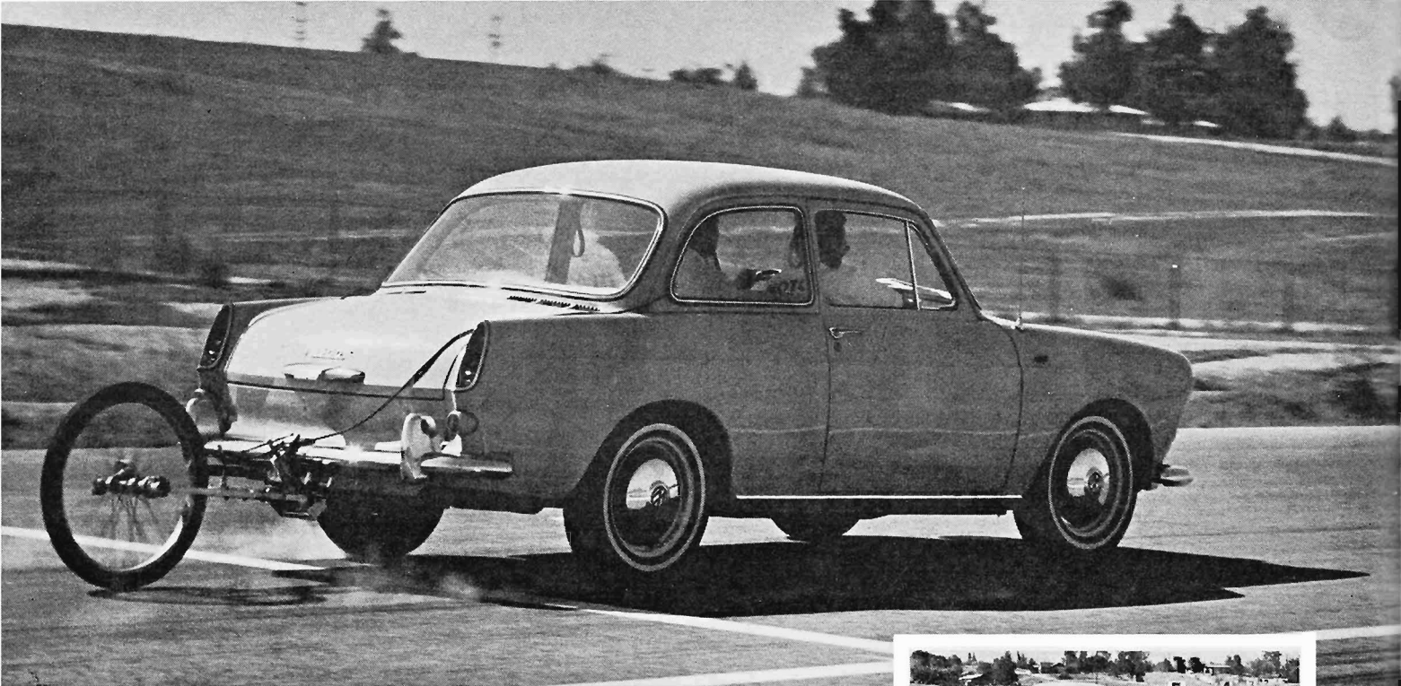
(ABOVE) Braking tests revealed how weight shift permitted rear wheels to lift and lock up first. Car remained under control during panic braking, stopped in a reasonable distance.
