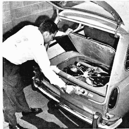
(ABOVE) Station wagon's engine nestles beneath insulated panel. Oil can be checked from external dipstick without opening engine. (TOP RIGHT) Two-door station wagon offers adequate rear seat space for passengers. Seat folds forward and flat (RIGHT) for long, open carrying area. Rear door swings upward, has fixed window. Wagon shouldn't be driven with door open, so lengthy objects can't be hauled as in some wagons.
