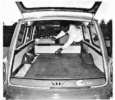
(ABOVE) Station wagon's engine nestles beneath insulated panel. Oil can be checked from external dipstick without opening engine. (TOP RIGHT) Two-door station wagon offers adequate rear seat space for passengers. Seat folds forward and flat (RIGHT) for long, open carrying area. Rear door swings upward, has fixed window. Wagon shouldn't be driven with door open, so lengthy objects can't be hauled as in some wagons.
