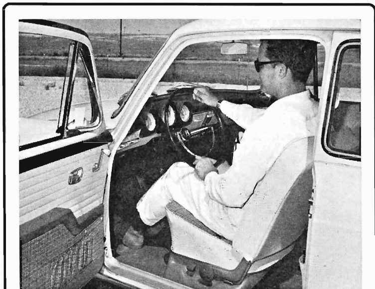
(ABOVE) Seating position in the 1500 is comfortable, offers good leg room. Seat has seven-position rake adjustment controlled by knob near seat base. (LEFT) Dash panel in 1200 is austere in contrast to 1500, with fewer instruments, no padding. Dash is functional, built for economy.
