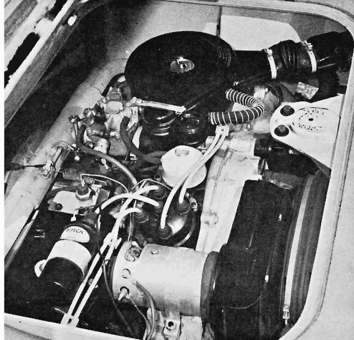
Engine for the 1500 is similar in design but has cooling fan driven off crank nose, is much quieter, forms flatter package.
