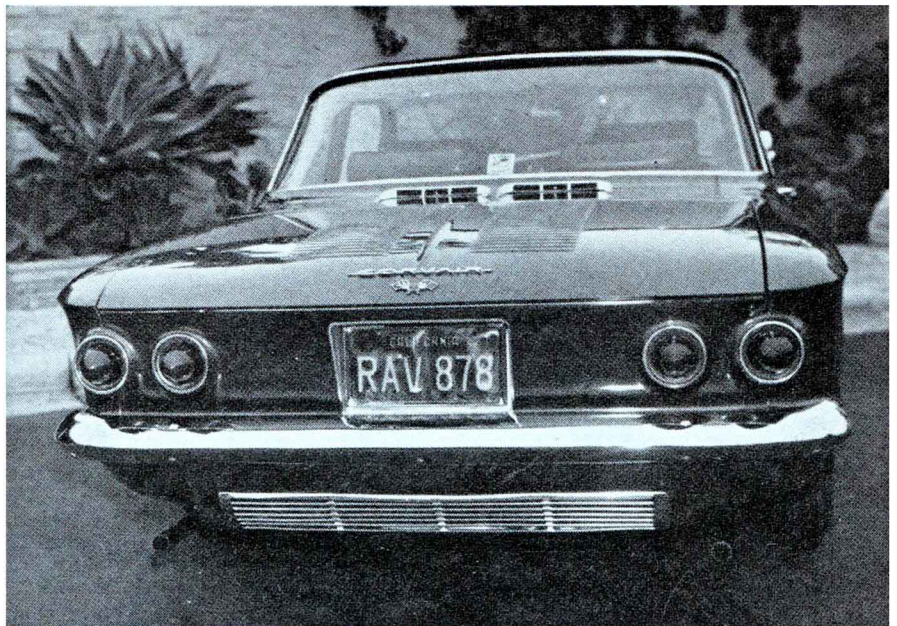
TWIN TAILPIPES of EMPI's Bestone system project from under Monza's rear.
