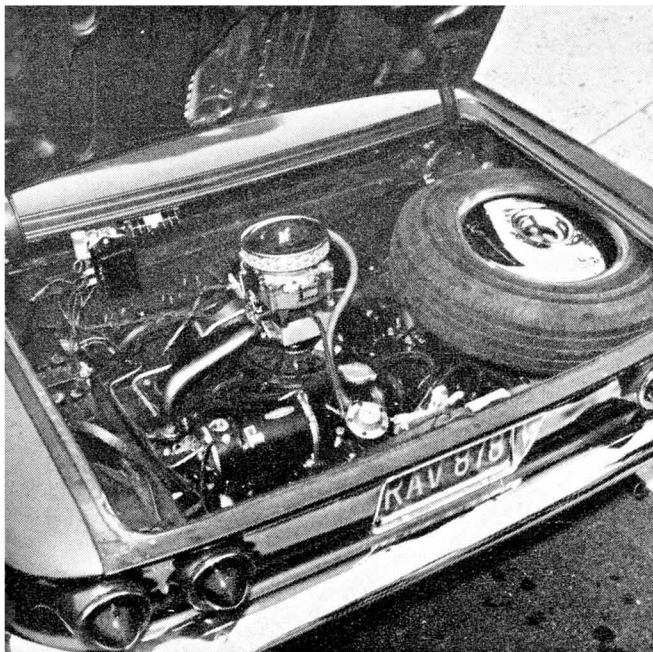
BIG CARBURETOR mounts on manifold extensions.
