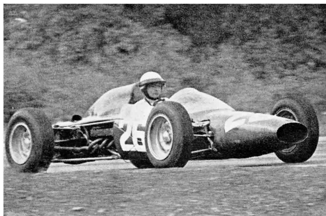
NEW ATS has conventional tube frame-chassis, V-8 engine.
