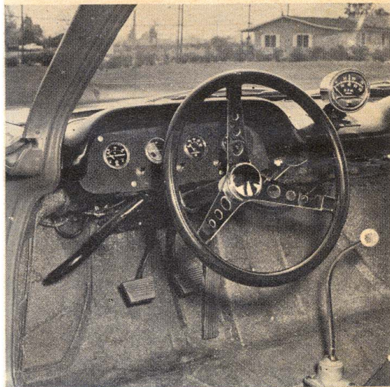
BELOW - Four gages in Going Corvair's instrument panel include two for cylinder head temperature and one each for oil temp and pressure.
