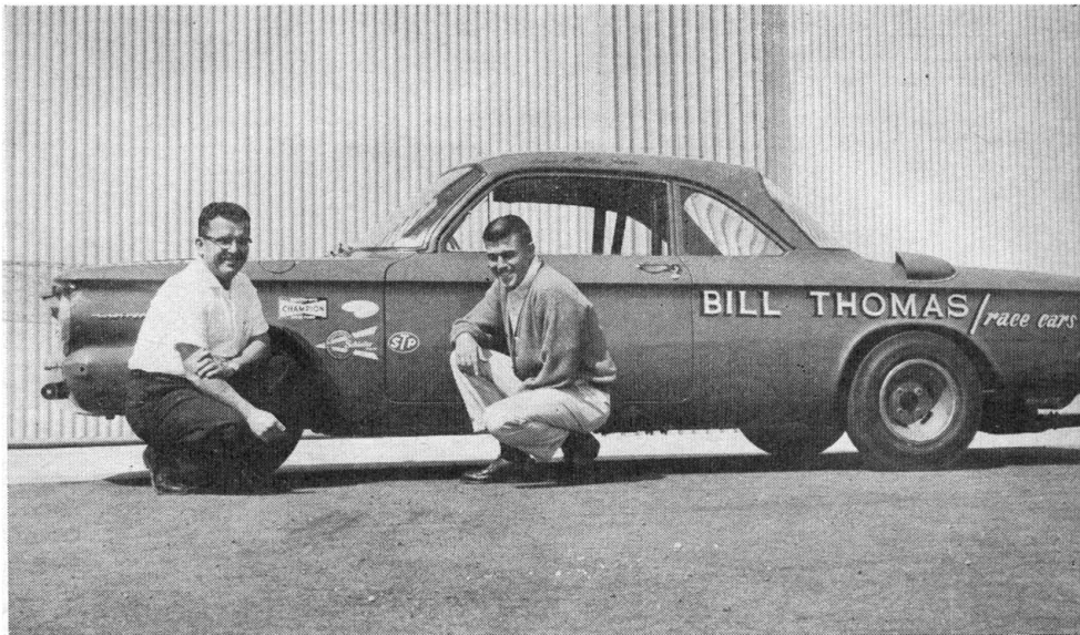
Standard front seat was replaced with a pair of upholstered fiberglass bucket seats that were mounted on tubular supports. Rear seat was removed completely. These changes alone reduced car's weight a little more than 100 pounds. Posed with their Riverside Red beauty are Bill Thomas, left, who owns it, and Mike Jones, who did most of the work on it and does all driving.
