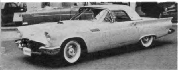
1957 Longer rear deck enclosed spare tire; power was supplied by 212-bhp engine.
