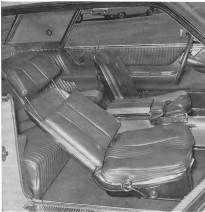
NOW YOU see it, now you don't! Door-side half of Thunderbird seat belts disappears when unhooked. An inertia reel next to the sill keeps things neat.
