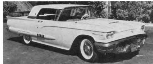
1958 First 4-passenger boasted larger, 352-cu. in. V-8, 300 bhp and unitized body.
