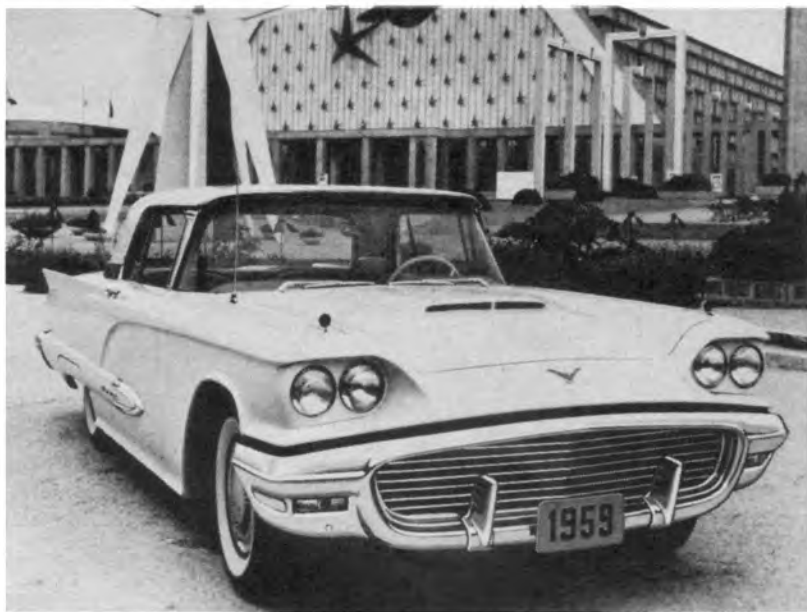
1959 Retaining the same shapes and sheet metal, this 'Bird had an interesting option: the 430-cu. in. V-8 now in Lincoln.
