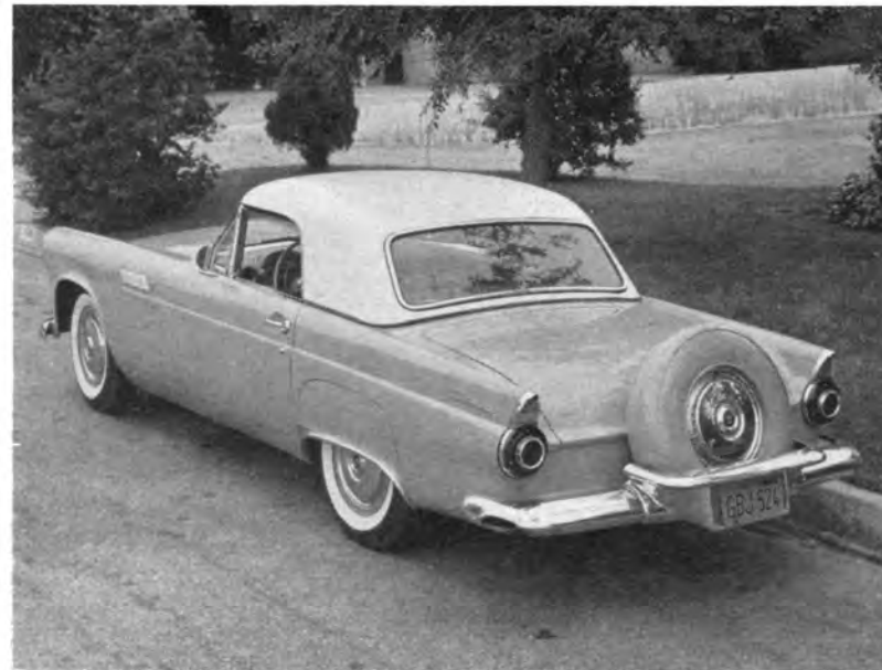
1956 Continental spare tire provided more luggage space. Optional hardtop also had "porthole" quarter windows.
