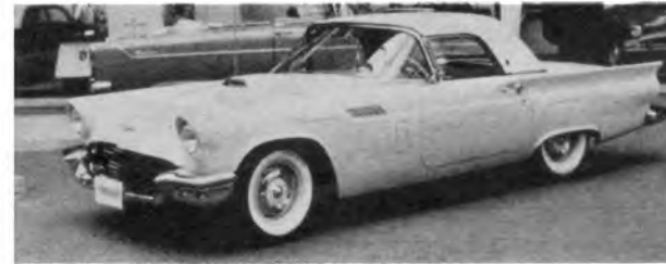
1957 Longer rear deck enclosed spare tire; power was supplied by 212-bhp engine.
