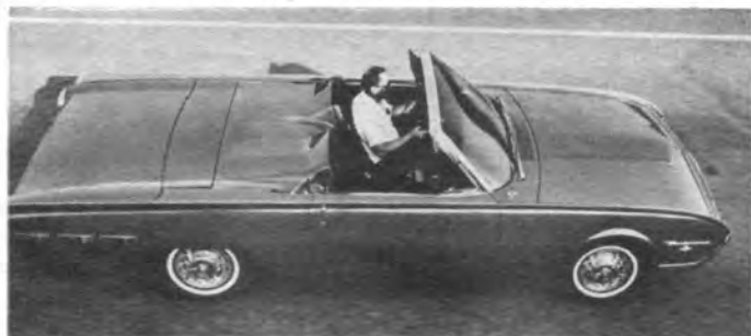
1962 Sports Roadster model was offered, included fiberglass tonneau cover, chromed wire wheels on convertible body.
