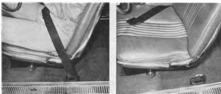
NOW YOU see it, now you don't! Door-side half of Thunderbird seat belts disappears when unhooked. An inertia reel next to the sill keeps things neat.
