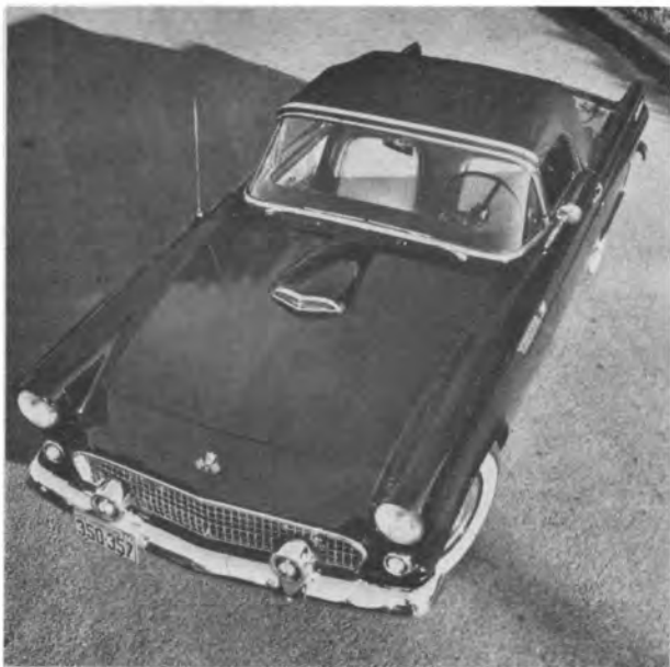
1955 First models appeared in both convertible and hardtop form; had 292-cu. in. V-8 for power.
