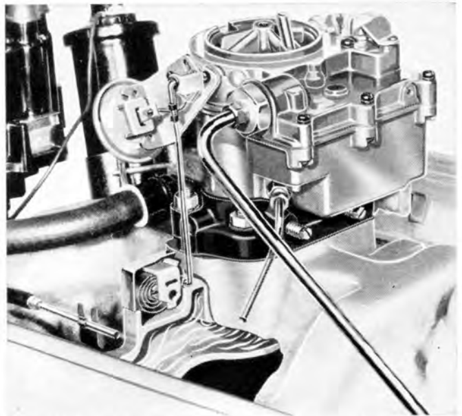
AUTOMATIC CHOKE on Chevelle has heat sensor in special heat stove cast in inlet manifold for quicker, more accurate choke response.
