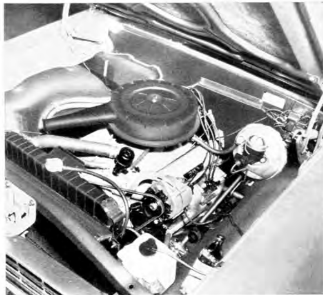
POWERING THE Chevelle is the 283-cu. in. Chevrolet V-8 rated at 195 bhp or, with 4-barrel carburetor and dual exhausts, 220 bhp.
