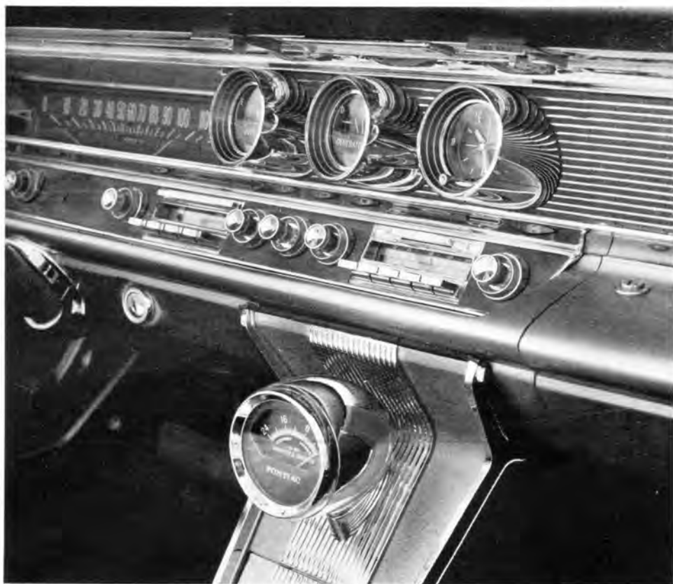
VACUUM GAUGE now mounts high on console in Grand Prix with automatic transmission.
