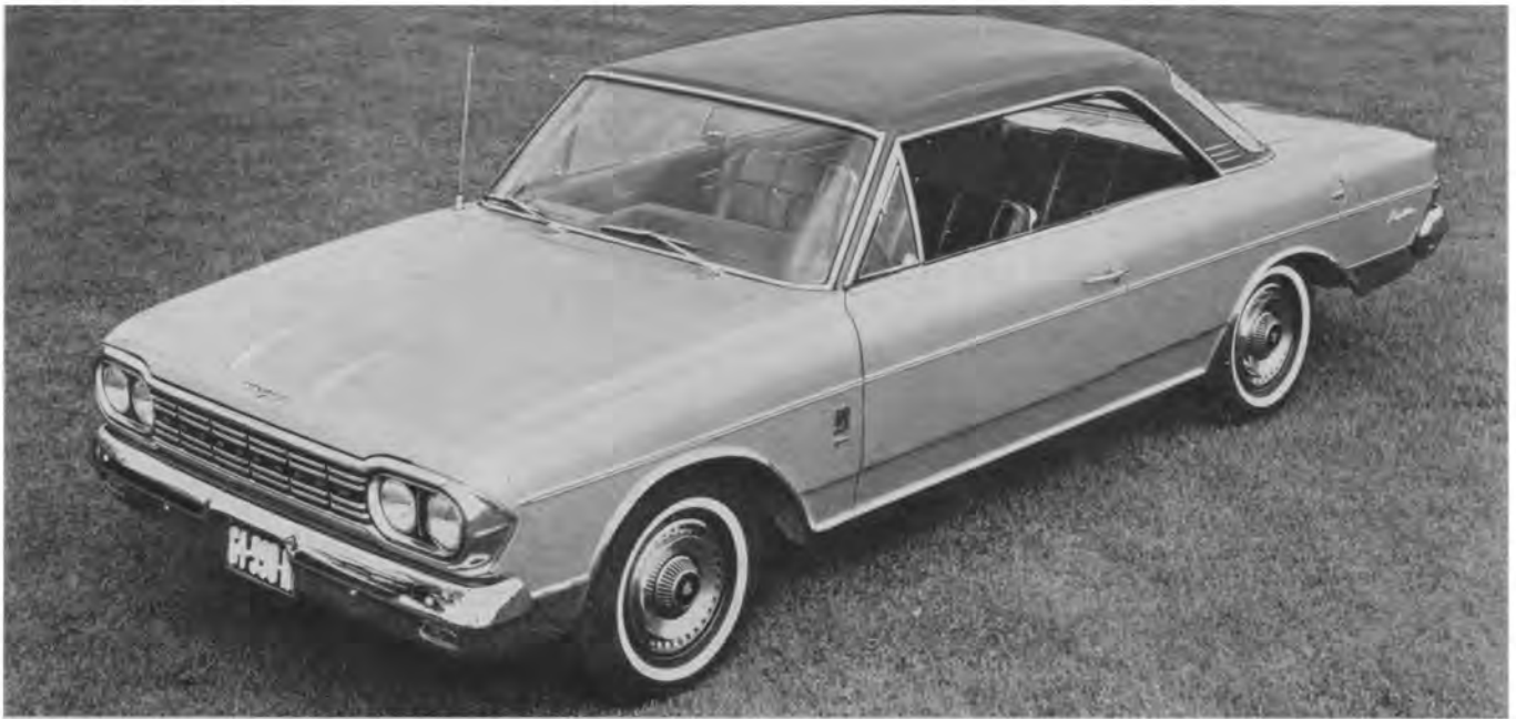
NEW HARDTOP ROOFLINE , shown here on the Ambassador, is 1-in. lower and is executed with classic simplicity. New grilles make front end less busy.
