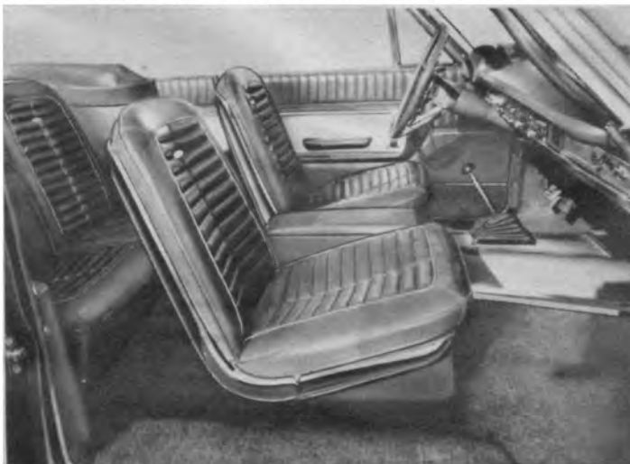
THIN-SHELL bucket seats are a new feature of the console-equipped Galaxie 500/XL series with all-vinyl interiors.
