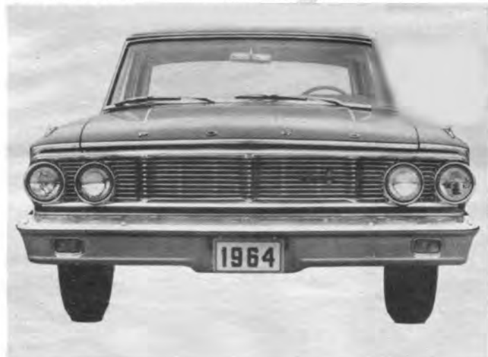
RECESSED grille bars on full-size Fords jut forward in three waves to give a three-dimensional appearance to the unit.
