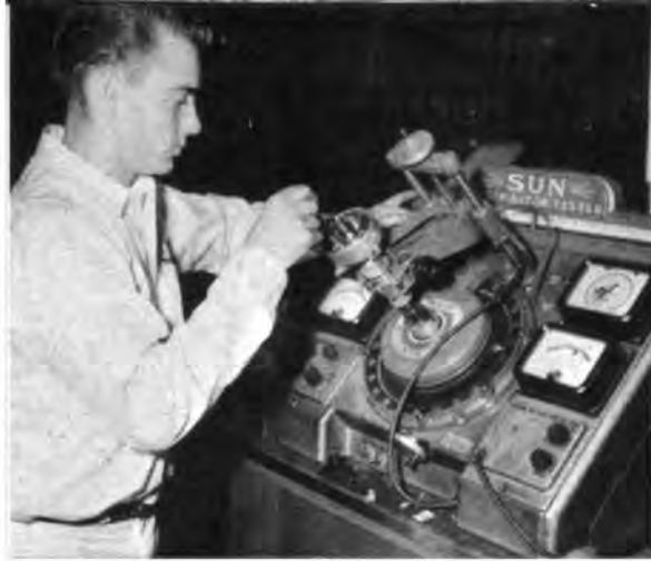
Fuel filter is removed (left) and the lines re-covered with aluminum foil to keep heat down. Bill sets up the distributor on the Sun machine (right) before buttoning the car up for a dragging day.
