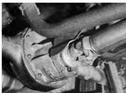
Detroit Automotive locking differential carries 4.86 rear gearing. It's a must for dragging and uses a raised pinion snubber for operation.
