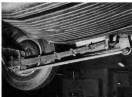
De-arched leaves have clips at rear. All rubber insulation was removed. Traction bars are by Les Ritchey. Springs have extra leaves. Big A-1 drag slick is compared to stock Galaxie rear tire, mounts on Holman & Moody safety wheel.
