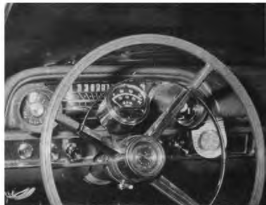
Extra bracket (left) secures lightweight 'glass hood in position. Hood would blow off without bracket. Sun tach goes to 8,000 rpm. Oil pressure gauge is at driver's right.
