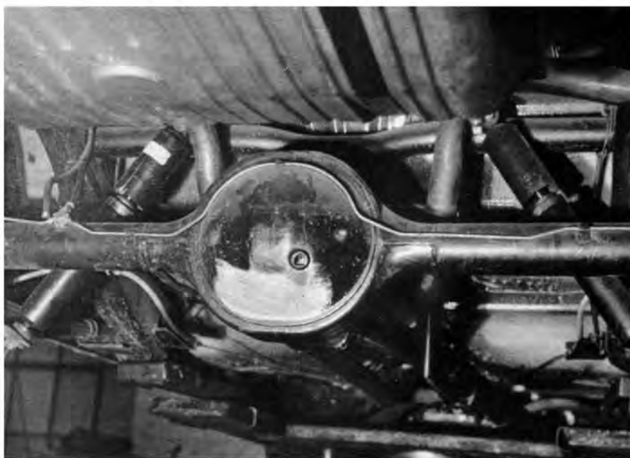
Detroit Automotive locking differential carries 4.86 rear gearing. It's a must for dragging and uses a raised pinion snubber for operation.
