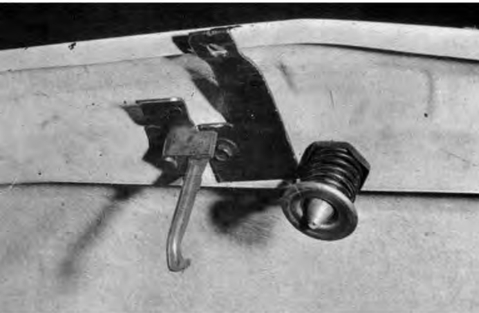
Extra bracket (left) secures lightweight 'glass hood in position. Hood would blow off without bracket. Sun tach goes to 8,000 rpm. Oil pressure gauge is at driver's right.
