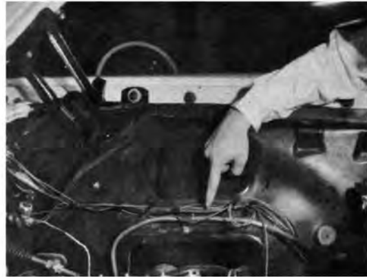
Fuel lines are relocated so that they aren't near most intense engine heat.
