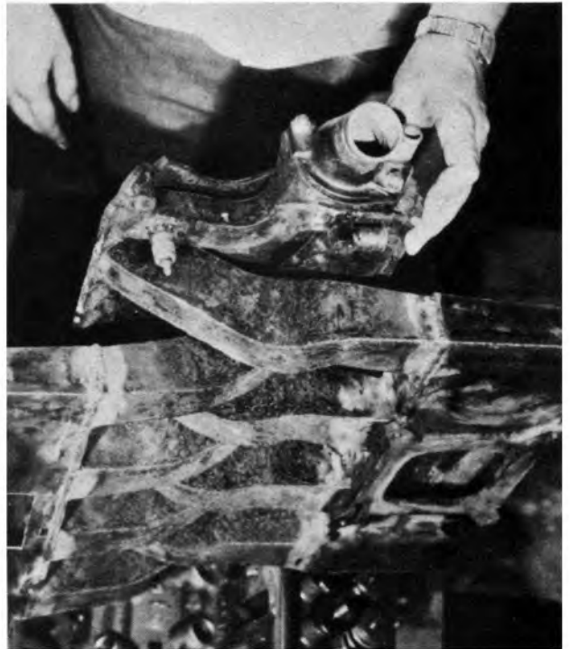
The stock water passage is duplicated in sheet metal but will be cast in aluminum when production starts. Use of wide plenum chambers makes it necessary to pull manifold when the rocker covers must be reached.
