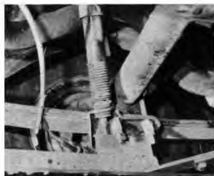
Traction bars of 1 X 3, .125-inch wall tubing measure eight feet and are welded to the rear spring pads. Bar at lower right is part of hoist.
