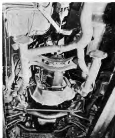
The four-speed transmission is used to accomplish 7,000 rpm shifts. The car storms through the traps at 6,500-7,000 rpm using a 5.43 rear end.
