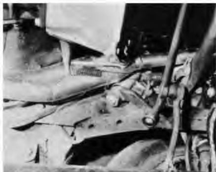
The long branch headers are routed along both sides of the clutch equalizer bar. This installation calls for some manual dexterity.
