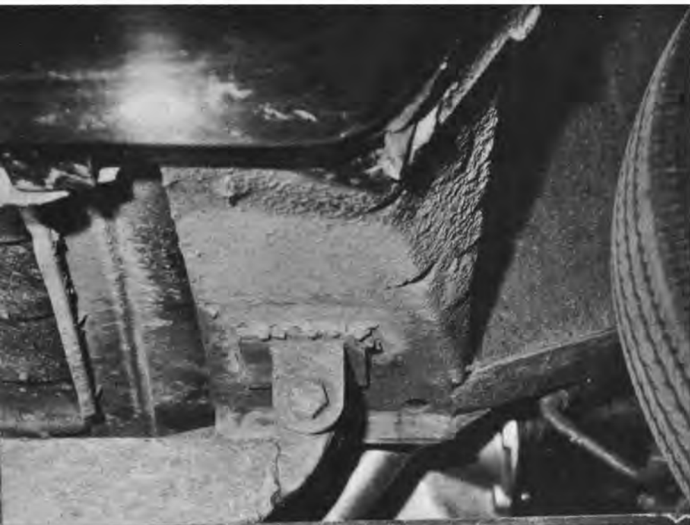
Traction bars up front pivot on the chassis and hinge on idler arm bushings. The plate welded to the car's floor pan acts to spread out the load.
