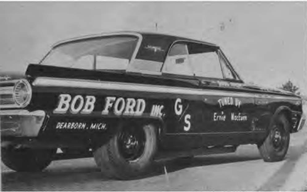
Hot 289 Fairlane fitted with headers and suspension changes has been cleaning up at the strip, is even faster with special ram manifold. Note long traction bars pivoted at front of chassis and extending back to rear axle.
