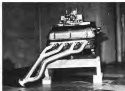
The headers have generous sweeps, but hug the contours of the engine and thus require nothing in the way of sheet metal modification.
