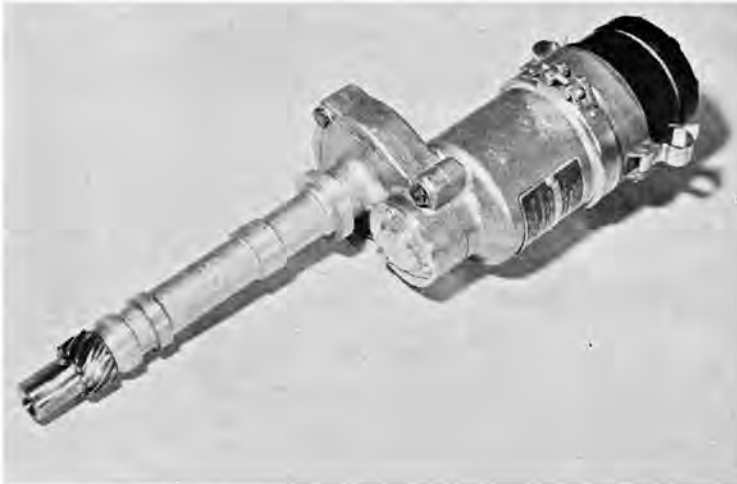
TOP - Crankshaft was cast ductile iron with 2.880 stroke for a 254.4 c.i. displacement. Total weight of crank, 48 lbs. BOTTOM - Mallory Mini-mag was special one with step-up gears so it could be used with Schaller quarter-speed cam. RIGHT - Counterweights added each side of center main.
