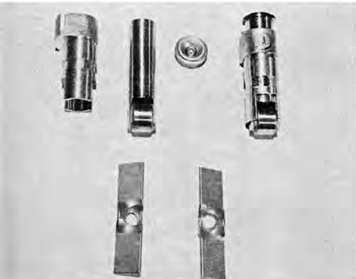
TOP - Schaller quarter-speed, double-lobe camshaft was the only shaft of many tested that would allow the engine to deliver enough power to make the race and to finish it. CENTER-Injector had long tapered passage, each cylinder. BOTTOM - Schiefer roller tappets and steel retainer straps.
