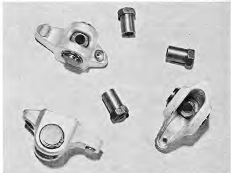
TOP - This double-row roller chain, driven by a sprocket bolted to the cam, drove engine fuel, oil and water pumps. CENTER - Rings formed from copper wire and installed in grooves in the aluminum heads improved gasket sealing. BOTTOM - Aluminum rockers rotated on needle bearings.
