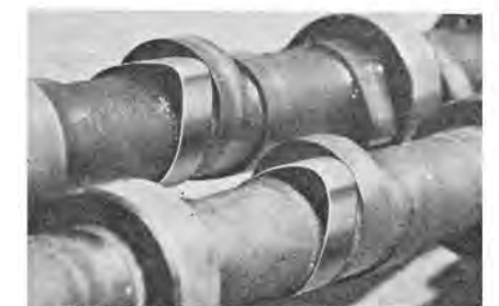
Big valves get heap big action via high-lift, long-duration cam (right). Note the difference between lobes on special stick and Falcon stock cam (shown at left).
