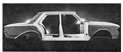
**ALL NEW!** Advanced Unit Construction. Major breakthrough in car construction replaces scores of small parts with massive uniside members, formed from one piece of galvanized steel (in white above). Stronger, longer lasting.
