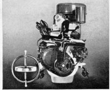
ALL NEW! Tri-Poised Power—vibration-free ride. Engine is 3-point seated in deep rubber!
