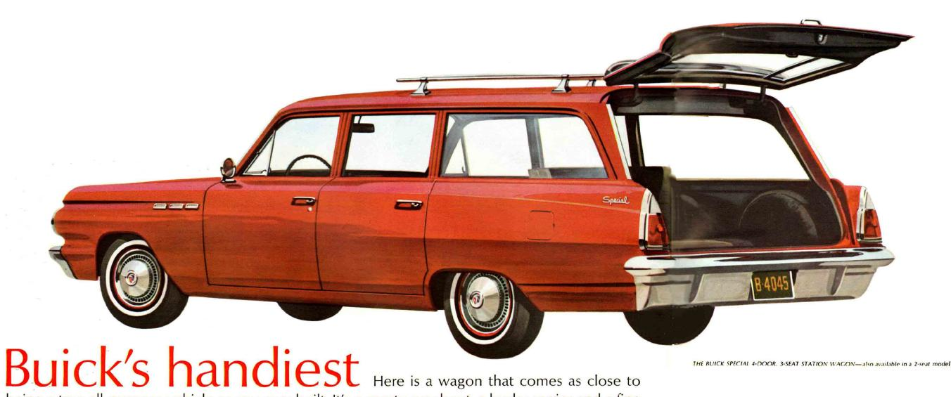
being a true all-purpose vehicle as any ever built. It's a sporty runabout, a husky carrier and a fine road car—all in one. Surprising, really, how much a Buick Special wagon can hold—almost 74 cubic feet of cargo. Loading is extraordinarily easy, too, with a full-height lift gate that swings up out of the way on counterbalanced hinges. You can take your pick of three Special wagons—4-door, 2-seat; 4-door, 3-seat; or deluxe 4-door, 2-seat. And you can power your wagon with any
