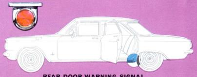
REAR DOOR WARNING SIGNAL Flashes ared warning light until both rear doors are properly closed.
