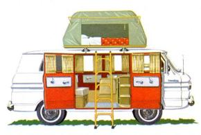
CAR TOP SLEEPER AND LADDER UNIT A durable waterproof sleeping unit that will accommodate a ¾ size mattress. A two section ladder is furnished with the unit.
