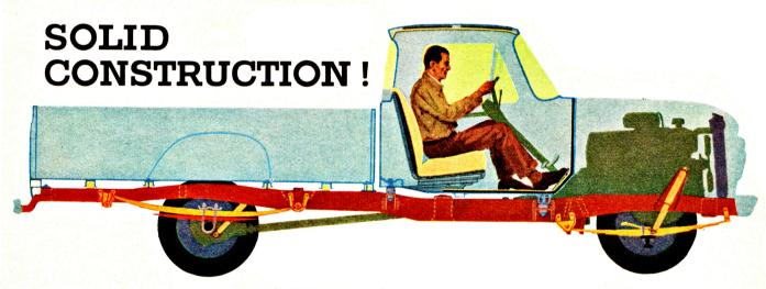
• Parallel-rail frame resists twisting; puts solid foundation under entire truck! • All-welded steel construction of both cab and box means less rattles.
