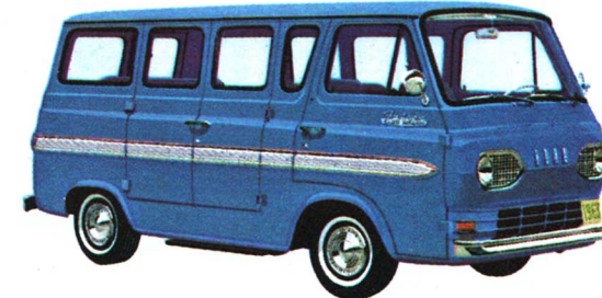
Extra-Duty Wagon Dimensions: Length 168.3"; Width 75"; Wheelbase 90"
