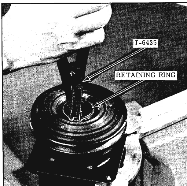
Fig. 15-47 Removing Pulley Retaining Ring
