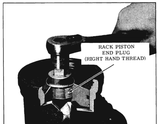
Fig. 4-251 Removing End Plug
