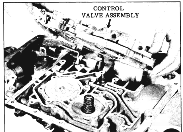
Fig. 3-317 Installing Valve Bodies
