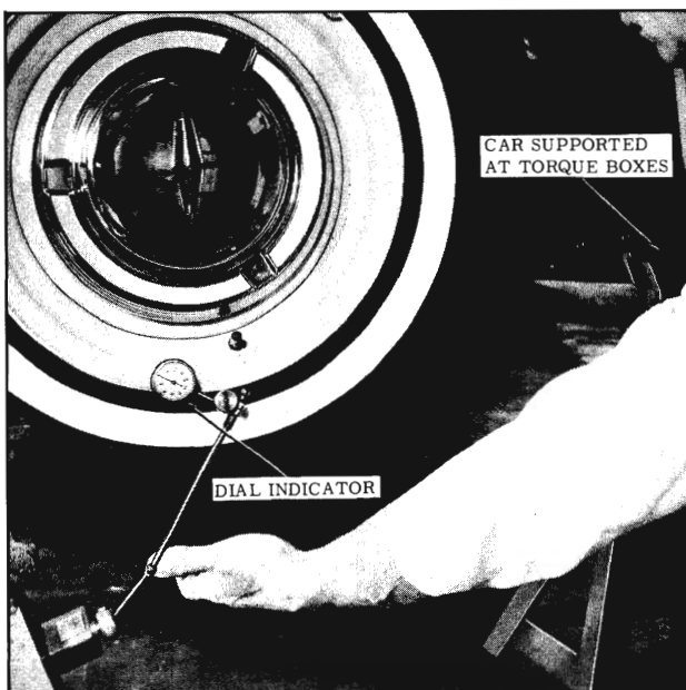
Fig. 5-17 Checking Lower Ball Joint
