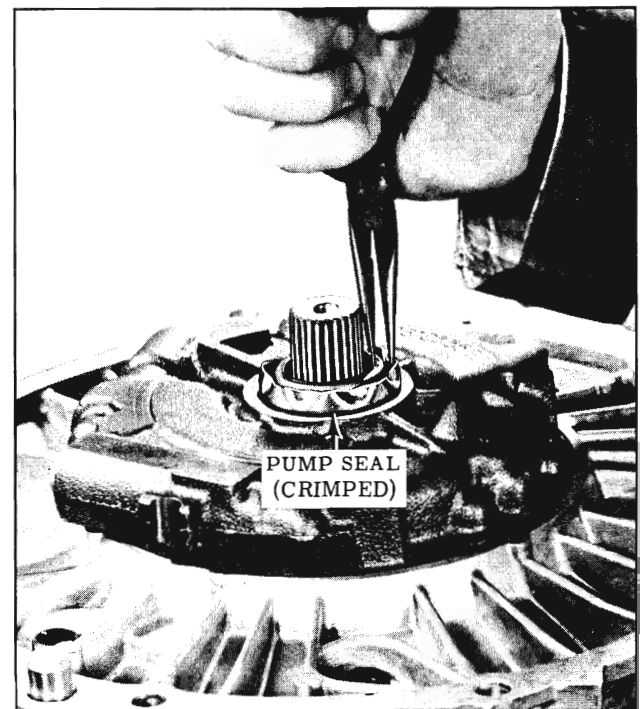
Fig. 3-237 Removing Pump Seal
