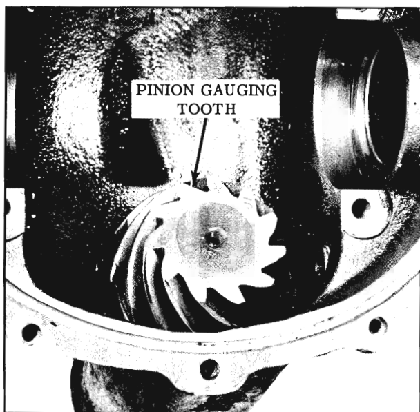
Fig. 6-127 Pinion Gauging Tooth
