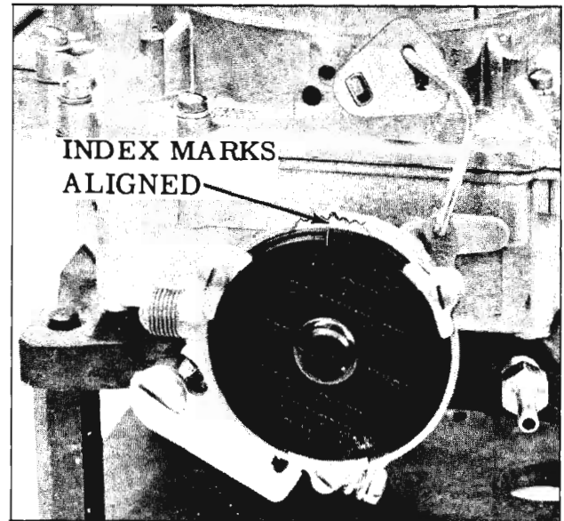
Fig. 9-24 Choke Coil Setting
