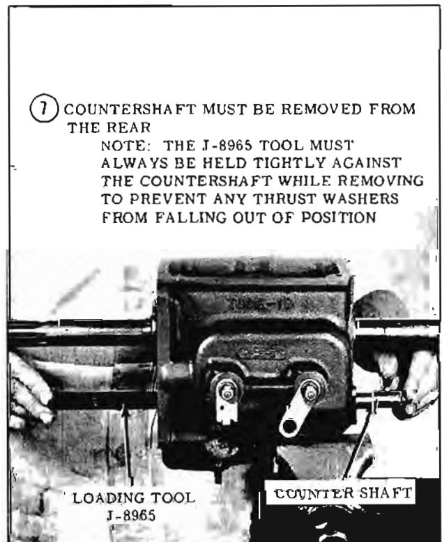
Fig. 11-117 Countershaft Removal
