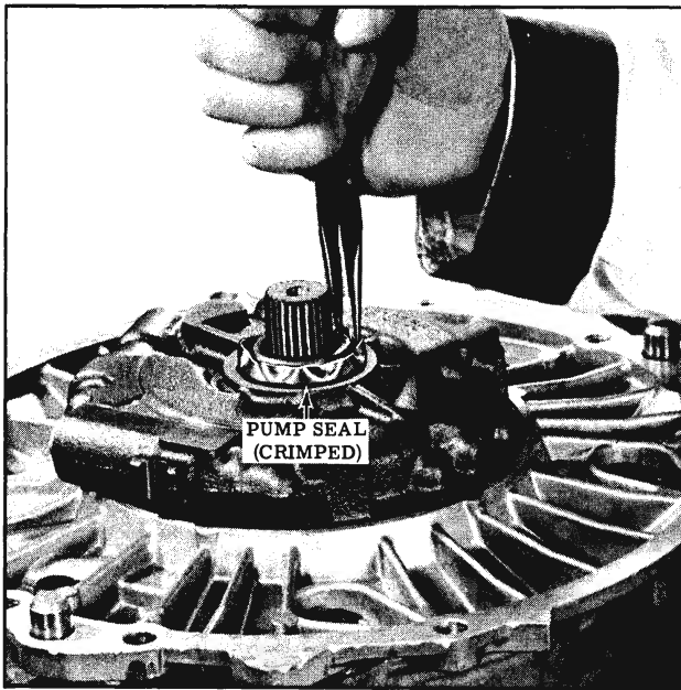
Fig. 3-31 Removing Oil Pump Seal
