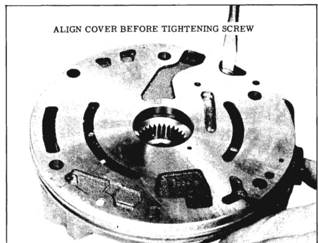
Fig. 3-57 Installing Pump Cover
