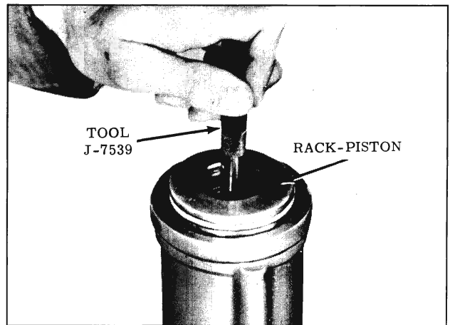
Fig. 4-253 Removing Rack Piston
