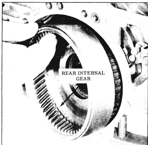
Fig. 3-43 Removing Internal Gear
