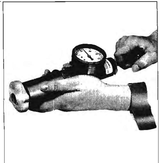
Fig. 8-172 Testing Fluid Tank Cap
