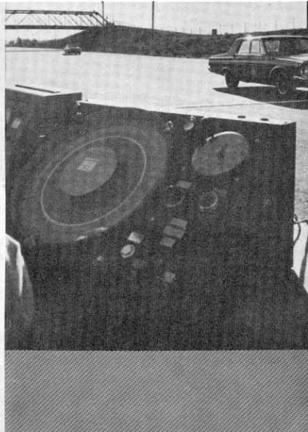
**ZERO-TO-SIXTY DRAG** This is a recognized test of acceleration from a standing start. For split-second accuracy, a light is attached to the roof of each car as shown in the photo below. Because of the variance in speedometers, a central electronic device is used to gauge the speed of each car. As the car reaches a speed of 60 miles per hour, the light blinks and elapsed time is recorded automatically. The cars competed one at a time, with a different driver in each car each time. Look at the
