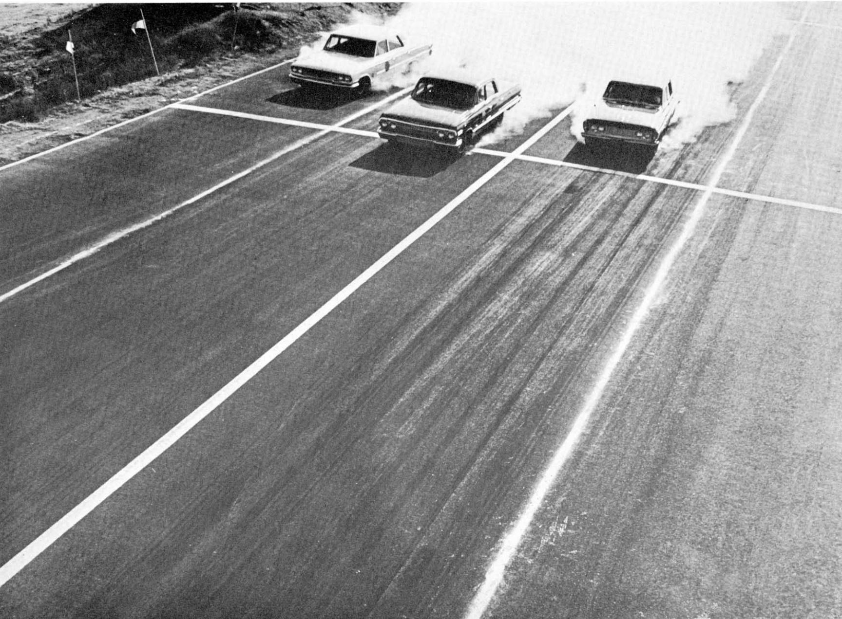
**ECONOMY RUN** Now it's time to put a price on all this performance. First, the gas is drained from each test car. Then, exactly two liters of regular gasoline (slightly more than half a gallon) are poured into a bottle for each car, and fed to the fuel pump through a hose. The drivers are instructed to maintain an average speed of 45 miles per hour, which means well over 60 mph on the straightaways to compensate for reduced speeds on the turns. As each car's engine dies, the driver
