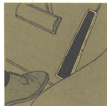
CRUISE CONTROL . . . automatically adjusts throttle setting to maintain speed you've dialed. A touch of the toe on the brake overrides automatic control. Eliminates foot fatigue on turnpikes. (D)
