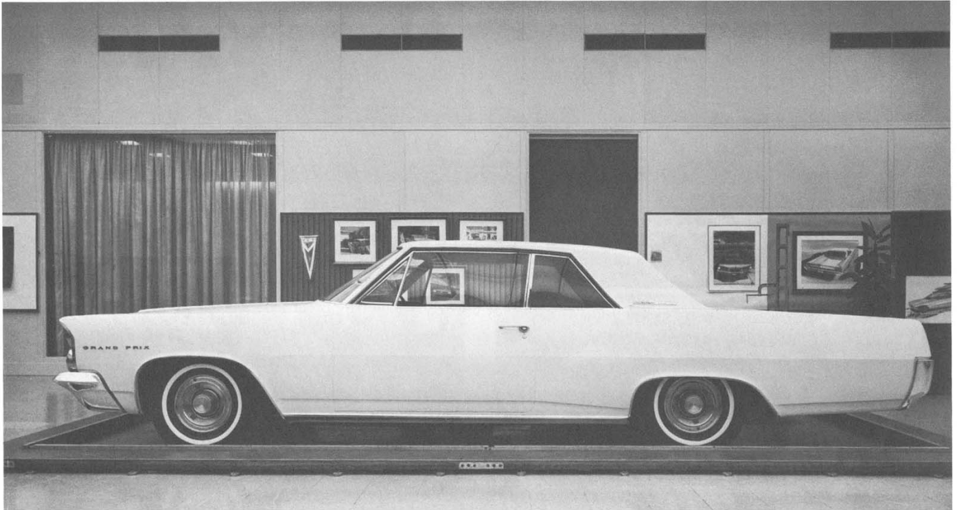
Like the final fitting for a dress, the fiberglass model of the Grand Prix is used to determine size, shape and placement of name plates and crests.
