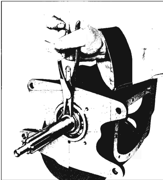
Fig. 7B-13 Removing or Replacing Main Drive Gear Snap Ring
