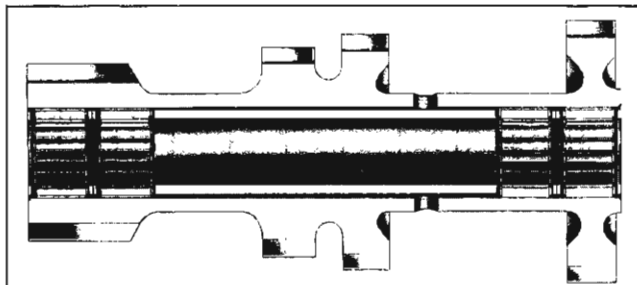
Fig. 7B-26 Cross Section of Countergear Assembly
