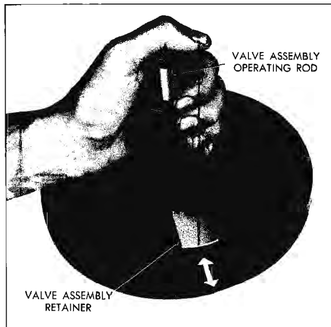
Fig. 5A-11 Removing Valve Assembly Retainer
