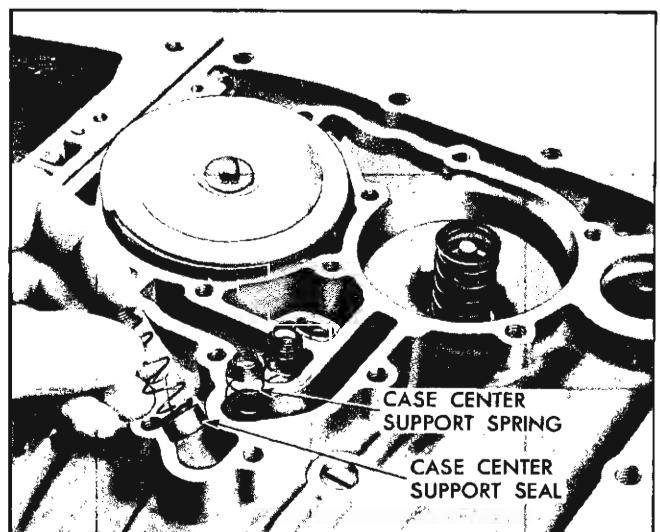
Fig. 7C-44 Removing Case Center Support Seals
