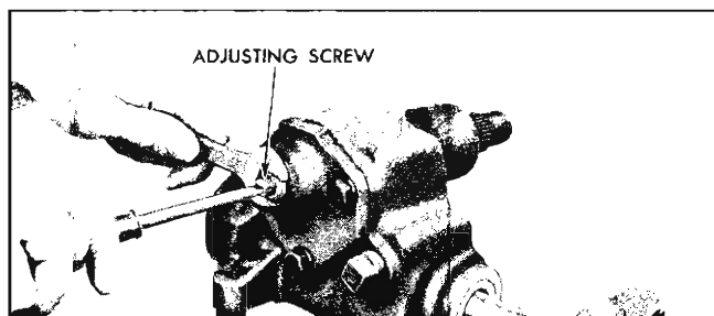
Fig. 9-4 Adjusting Pitman and Ball Nut Backlash
