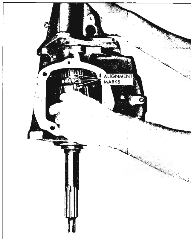
Fig. 7-37 Installing Mainshaft in Transmission Case
