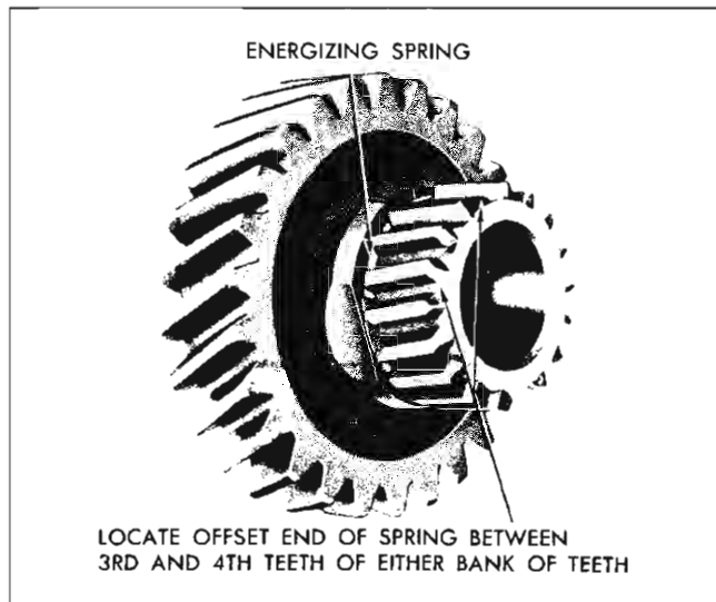
Fig. 7-28 Position of Synchronizer Ring Energizing Spring
