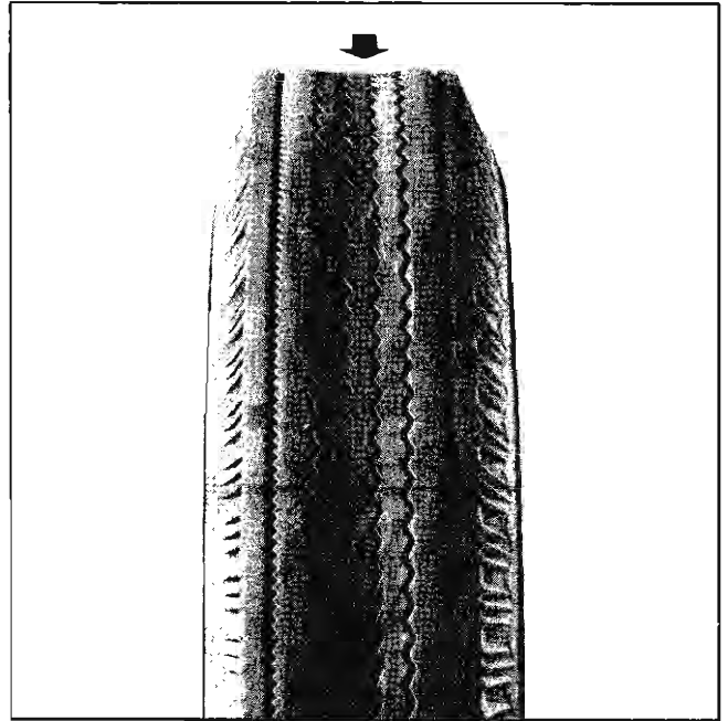
Fig. 3A-5 Wear from Overinflation
