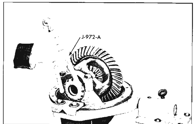
Fig. 4-20 Turning Adjusting Nut with J-972-A
