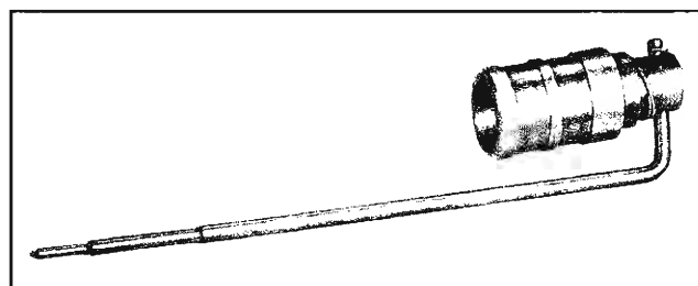
Fig. 6B-102 Step Up Rod and Piston Assembly
