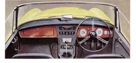
Essential for high-speed travel, the easily read instruments are closely grouped in a wood veneer panel in front of the driver. A short central gear lever in the console permits effortless changes and for driving comfort, the 17 inch diameter steering wheel has spring-spokes. A hard-wearing carpet over the entire floor completes the stylish interior trim.
