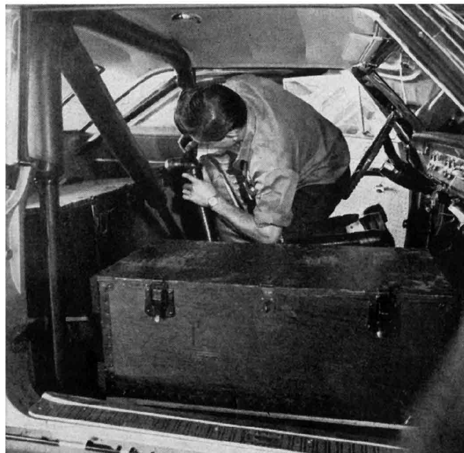
ROLL CAGE, wooden crates for spares and tools were installed in preparation for 6-week run.
