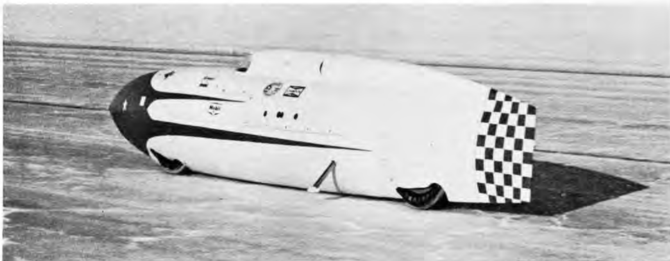
ABOVE—Pointed tail of Mangham-Alen Chevy-bike keeps air turbulence down at high speeds. Outriggers are used for balance on starts and stopping.
