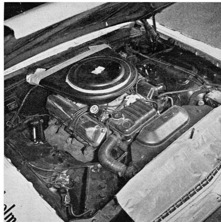
AIR CLEANER draws fresh cool air from cowl duct; tape on top of distributor keeps high tension leads from vibrating loose.
