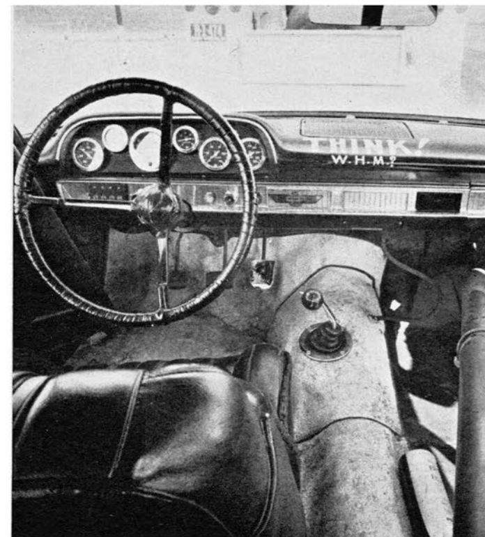
DRIVER'S VIEW includes oil and water temperatures, fuel and oil pressures, big electric tachometer and a reminder.
