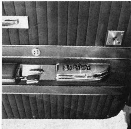
POWER WINDOW switches nestle on left door mount below remote mirror lever.
