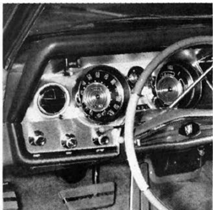
CRUISE-CONTROL lever operates vacuum and electric device which maintains set speed.
