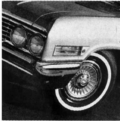
TURNING light on front corner lights up when turn signals are engaged.
