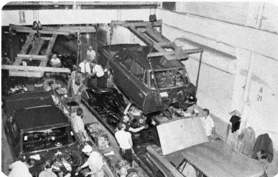
AT BODY DROP , completed shell from second floor meets up with chassis and engine on ground floor for final assembly. Front section is readied for drop moments later.
