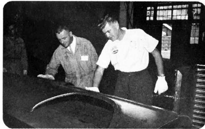
PRESS SHOP supervisor shows the novice how to detect flaws in finished stamping by rubbing gloved hand over surface.
