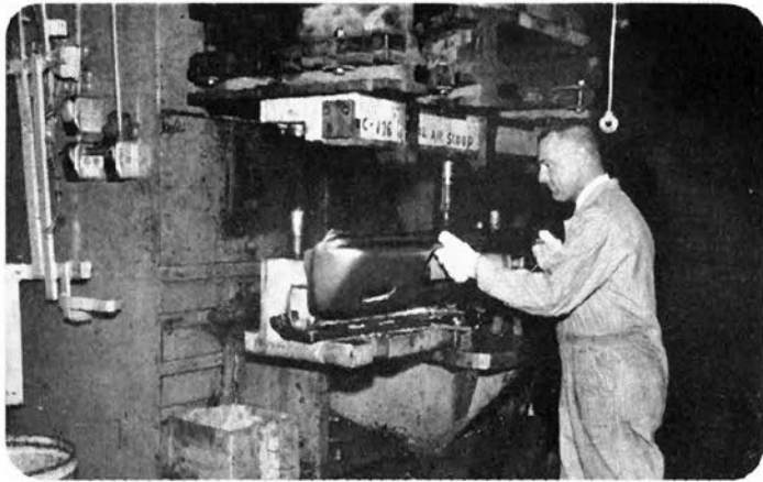
AMIDST HUGE presses, sheets of steel are bent into body parts with crimps, cuts and bolt holes automatically made.
