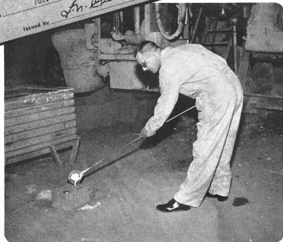
WHEN YOU BUILD your own car, the place to start is in the foundry where you draw a sample of the molten iron to test for hardness by molding a small sliver.
