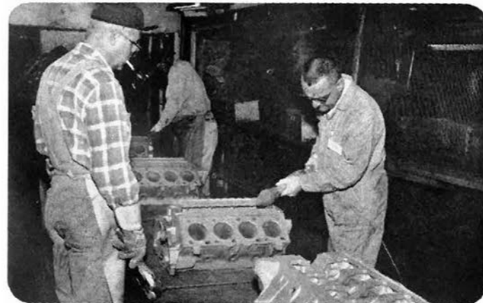
COOLED AND cleaned up, new blocks get the roughest edges chipped off and ground down before they move to the machine shop.
