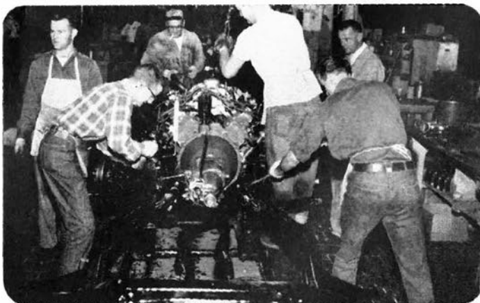
RED AND chrome R-4 engine is dropped in place onto heavy-duty chassis, which had been built up on another synchronized line.
