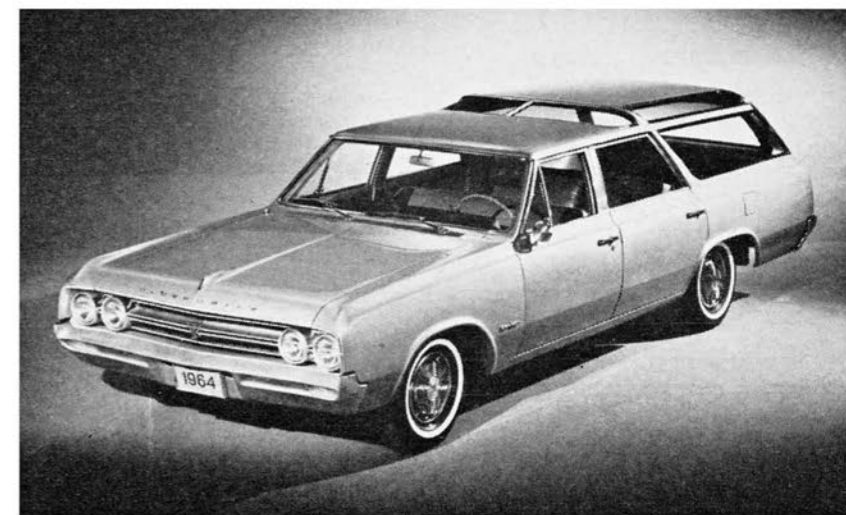
WHEELBASE has been increased 5 in. and rear door widened to accommodate the three forward-facing seats in wagons.
