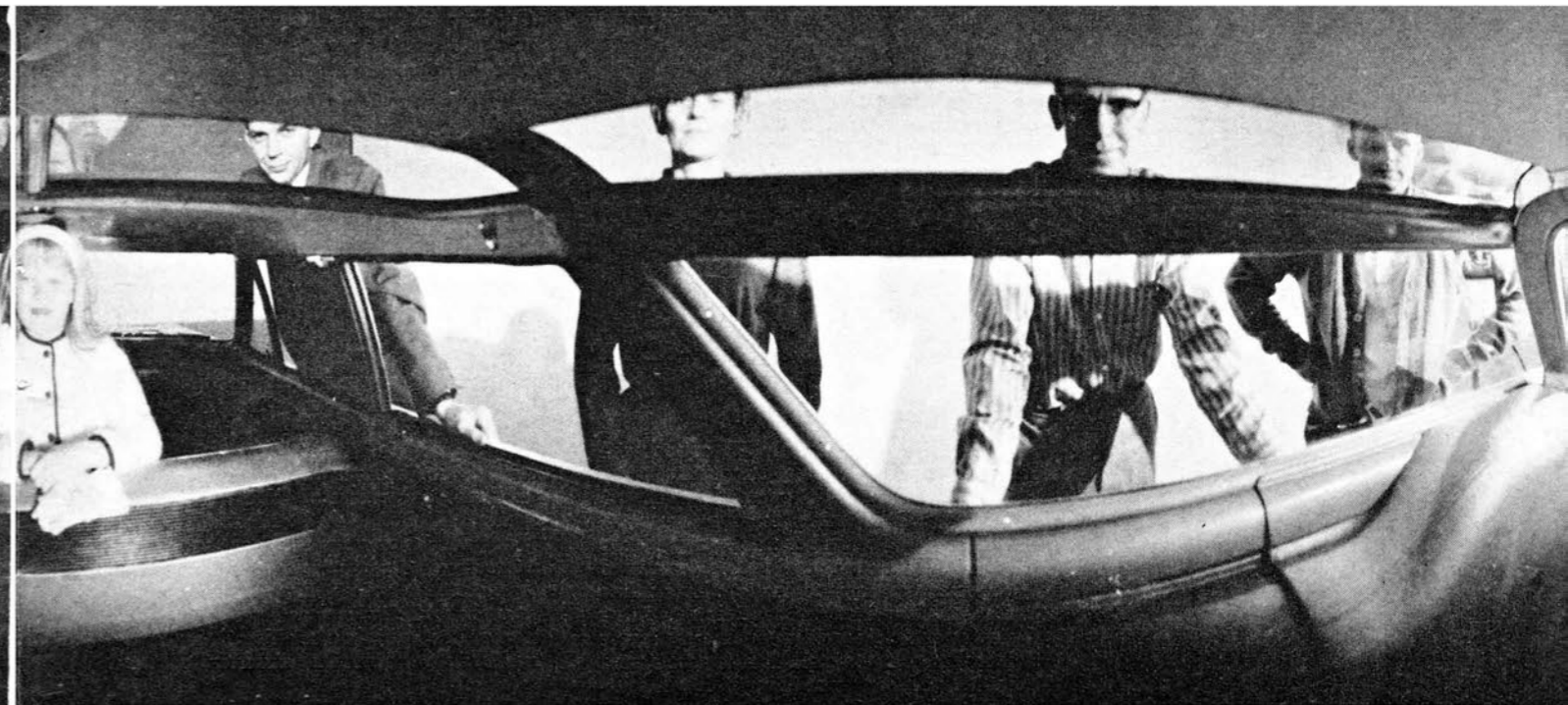
SPECIAL CAMERA viewing a full 360 degrees snaps the view a swivel-necked third seat passenger would have in the new Oldsmobile Vista-Cruiser wagon. Upper view-ports and windshield are tinted and heat-resistant.
