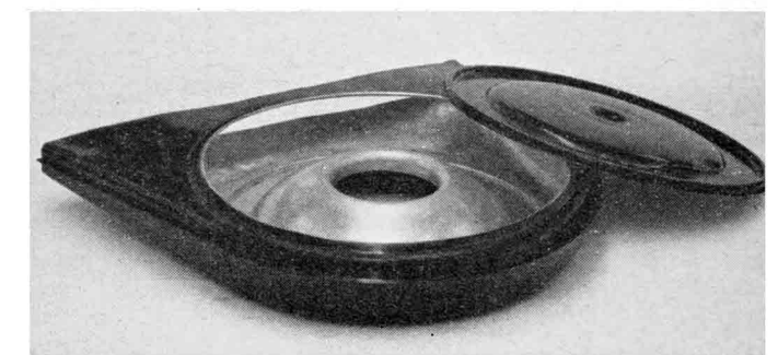
SPECIAL AIR intake chamber is designed for smooth, easy entry of ram air at 160-plus mph. SLIGHTLY exaggerated dotted lines show how cylinder bores are scalloped for better airflow with oversize valves.
