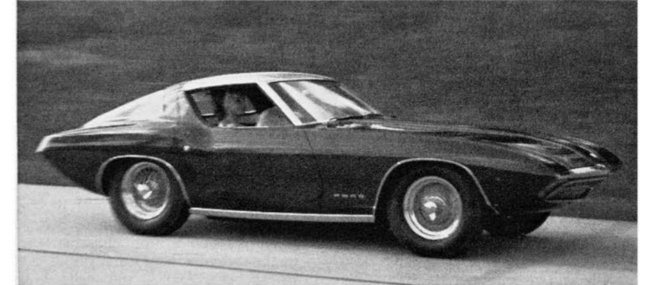
COUGAR II at speed has lean and ferocious look which delights enthusiasts. An unusual feature is panel between taillights which opens to relieve interior pressure.
