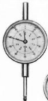
Model B, Right, Range of .400" calibrated in .001". Easy to read dial of .040" per revolution. Includes tolerance marks.
