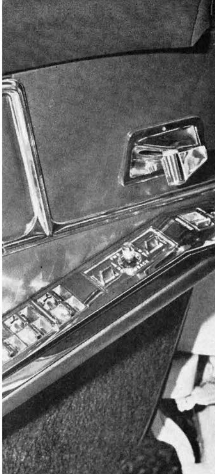
Switches for doors, windows, and seat are all grouped where driver can get at them.
