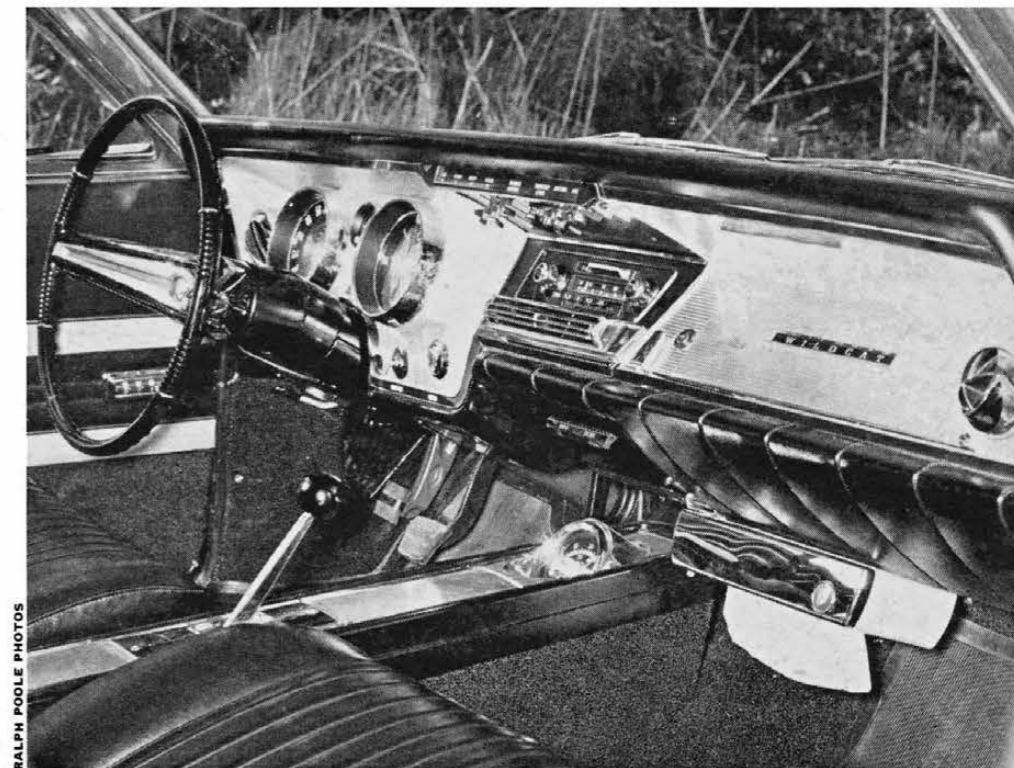
TWIN, HUGE dials enclose speedometer and other instruments. Forward-slant on shift lever makes it less easy to use; tachometer is nearly invisible.
