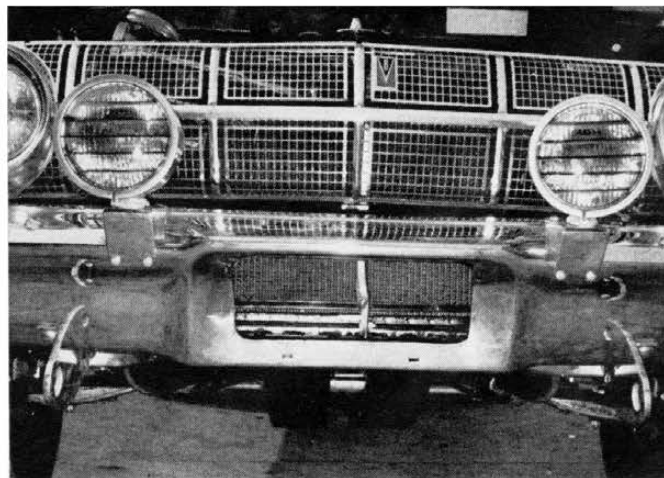
SPRING-STEEL skid plates extend back under engine and transmission. Extra lights are for foggy conditions.
