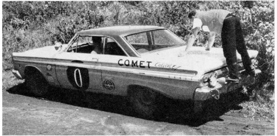
CO-DRIVER demonstrates his position when the driver calls for more traction; step plates on the bumper and handles on the deck help him keep his balance.
