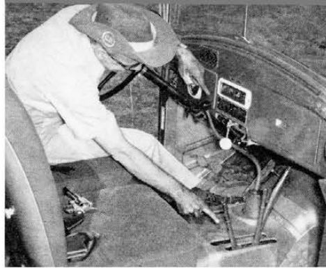
SHIFT LEVERS were designed for the wear-and-tear of competitive work. Lower set of sticks stirs up the transfer case and front-wheel-drivers.
