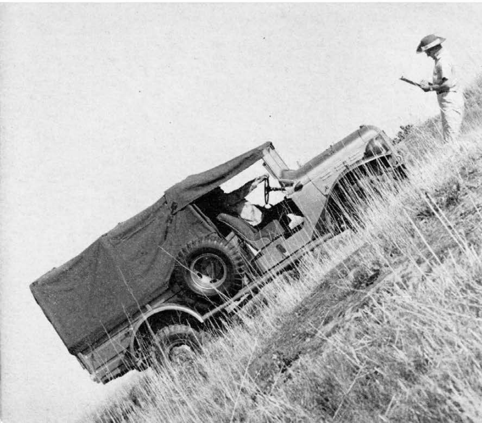
GRADABILITY IS EXCELLENT in both 2-wheel-drive and 4-wd. In 4-wd, with Grandma (low transfer) engaged, it seemed as if it would climb Kilimanjaro. Best-suited for the more rugged circuits, the Safari SS no doubt could distinguish itself in World Championship rallye events.
