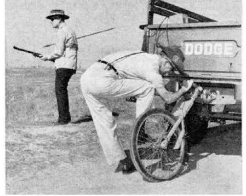
HOOKING UP THE eighth wheel to assure accuracy of speedo calibrations and the acceleration runs. The natives were beginning to get a bit restless.
