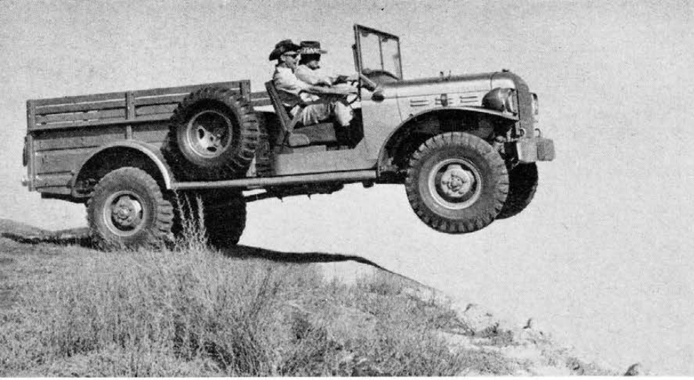
AGILE AS A mountain goat, the Safari SS fairly bounds over little rocks and rills. With strong suspension, leaps like this were commonplace and not harmful to our test car. Tires are max. traction 9.00-16 8-ply militaries, best suited to mud, flood, snow and other workaday situations.
