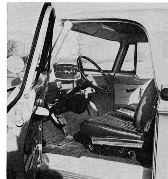
Interior uses Dart GT bucket seats and console, with carpets covering floor and gas tank. Steering wheel could be lower.
