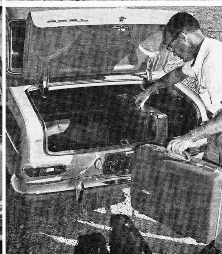
3) Spare and gas tank stand at sides of wagon cargo area, and floor lifts up to give access to added storage space beneath. 4) Sedan's tank is also inside fender, so there's enough room for five generous-sized suitcases plus smaller odds and ends.
