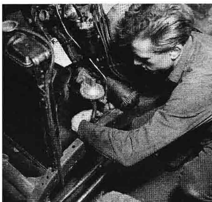
Note line being connected to the stock pump. Dual electrics are at the rear.
