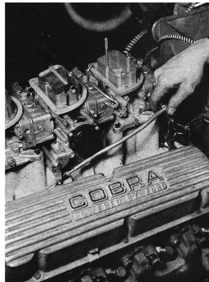
Bolt the plate over the opening at the rear of the aluminum manifold. Kit does not include vent plate, you must salvage it from the stock manifold. Next, connect the main carb arm to suitable linkage. Mechanical bell crank and linkage are cheapest.
