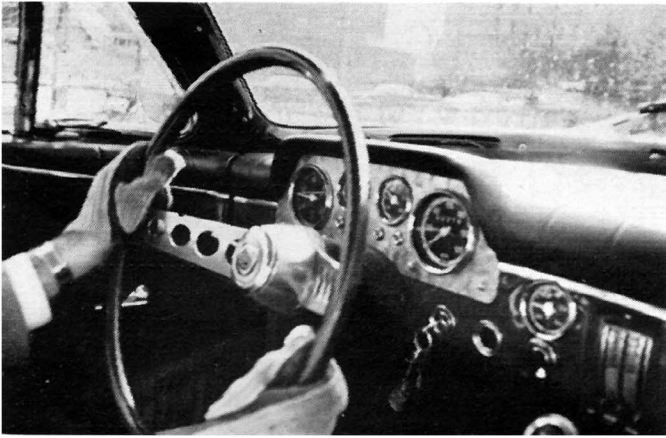
Steering wheel spokes are drilled for lightness; instrument panel is fully reworked, with great VDO dials for everything.
