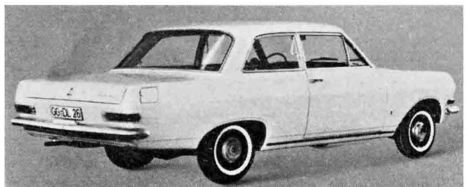
KADETT'S SQUARISH rear encloses a generous, for its size, trunk space. Vertically mounted spare and fuel tank help get usable space. Below, Kadett's more handsome big brother, Rekord.
