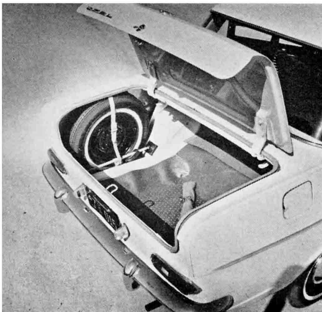
KADETT'S SQUARISH rear encloses a generous, for its size, trunk space. Vertically mounted spare and fuel tank help get usable space. Below, Kadett's more handsome big brother, Rekord.
