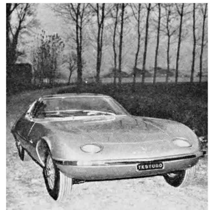
LUGGAGE FITS under front hood. Car is 169.4 in. long, weighs only 1980 lb.
