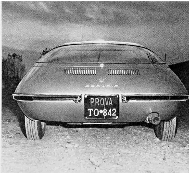
AFT VIEW shows why it was nicknamed "Testudo." Overall height is only 41.8 in., overall width only 67.8 in.
