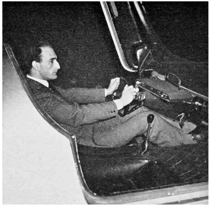
DRIVING POSITION is typically Italian—arms straight out, driver nearly reclining. Rectangular wheel might hamper cornering, though.
