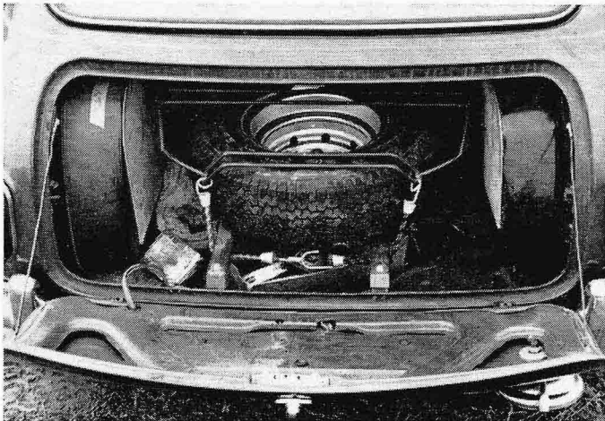
Spare tire in the Mini is held by a quick-release spring clamps.
