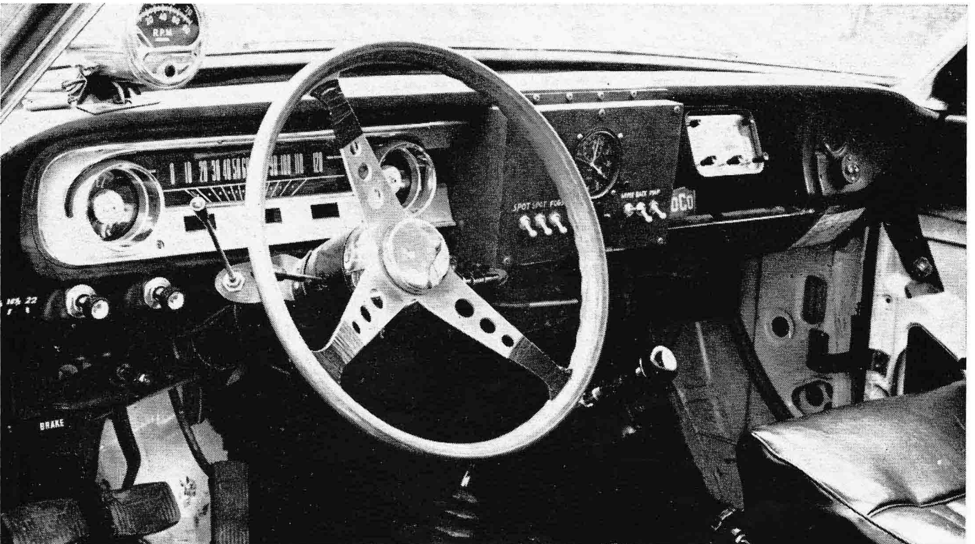
The Falcon's tachometer is unobtrusively located in corner of windshield; co-driver put trust in both clocks and Halda Speed Pilot.
