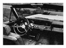
simulated wood grain overlay under a padded lip. The new round steering wheel has the Saginaw tilt option, with or without power assist, and reclining bucket seats permit a wide adjustment.
