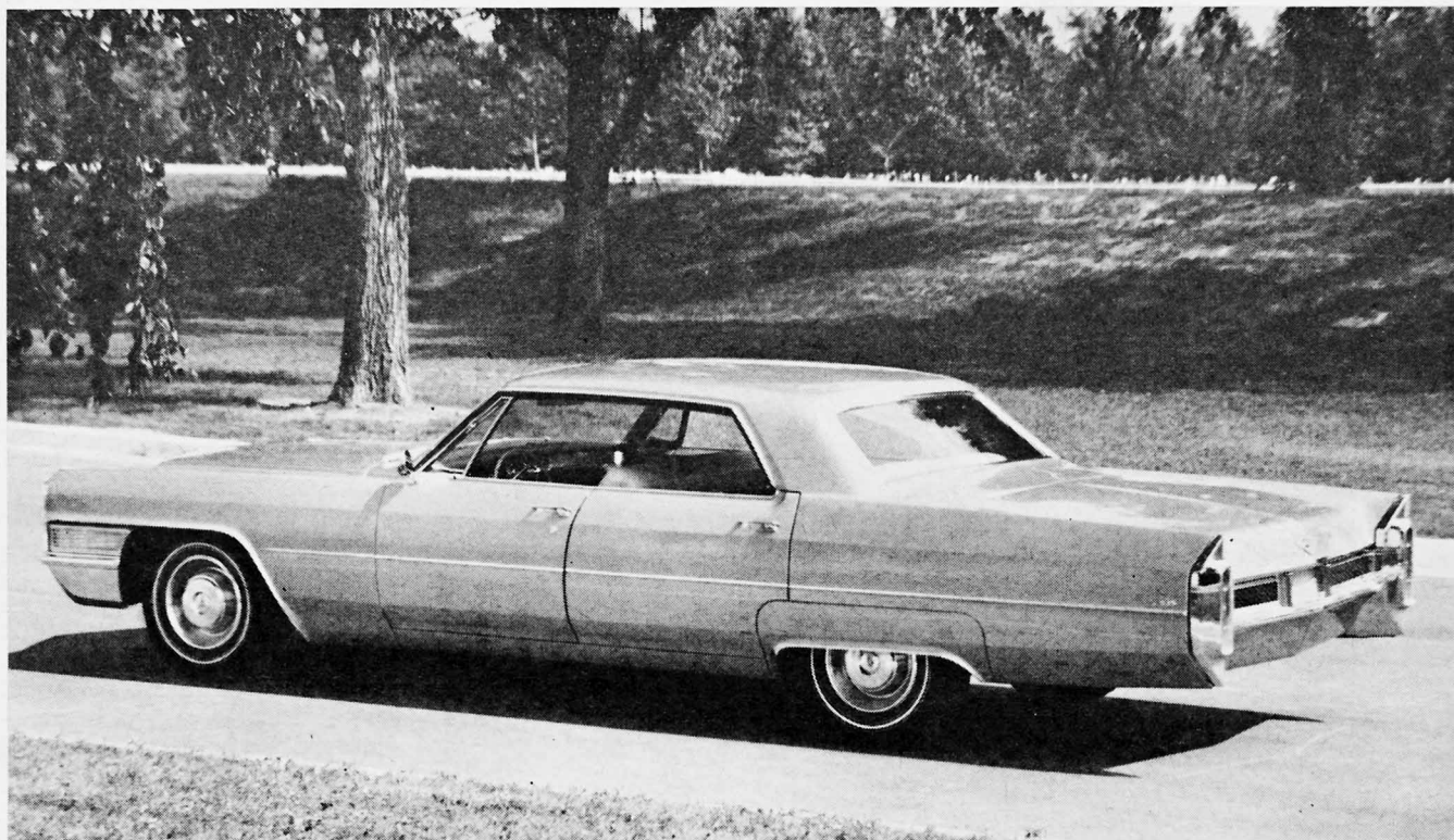
TULIP-TAIL styling let Cadillac dispose of traditional, 14-year-old tail fins gracefully by continuing the hint of fins. Side sheet metal styling is a distinctive 3-plane design and roof lines have been softened.
