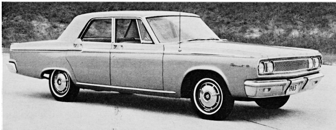
FOUR-DOOR SEDAN in the Coronet 440 series makes use of existing bodies with new front and rear-end styling to achieve smaller overall dimensions.
