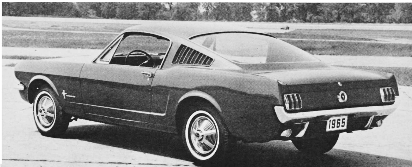
LARGE GLASS area of rear window extends from mid-roof to trunk opening and lack of curvature in the glass cuts down tendency to distort vision. Little else in Mustang styling has been altered for autumn announcement.
